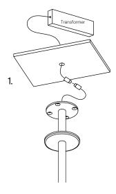
Prep the ceiling with an approx. 5-15mm hole. Place the transformer in the ceiling and feed the cable through the hole into the room. Connect the single electrified cable to the transformer.
