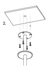
Screw the mounting plate to the ceiling using appropriate fasteners for the ceiling substrate.
