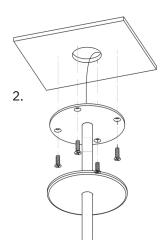
Screw the mounting plate to the ceiling using appropriate fasteners for the ceiling substrate.
