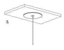
Flip up springs and fit through 60mm hole. Release springs to secure plate around ceiling substrate. (Maximum weight loading 1kg)
